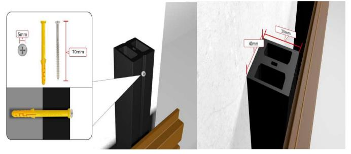
The composite josits are fixed by expansion screws, which goes into the wall for about 50mm (deducting the joist thickness).
