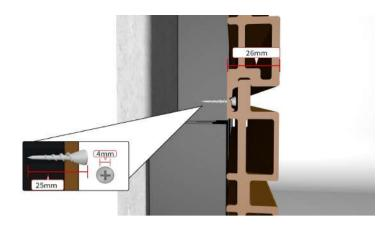
The groove should in the low postion and the tab in the high position.
